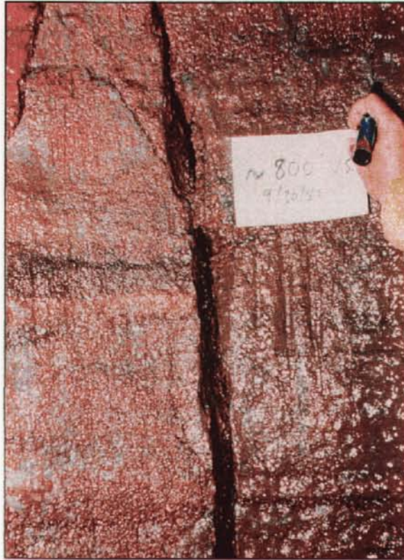
Plate 1. An open fracture in the unnamed lower member of the Rustler Formation.
